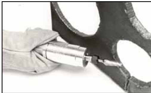
Front exhaust blows chips away from the operator.
