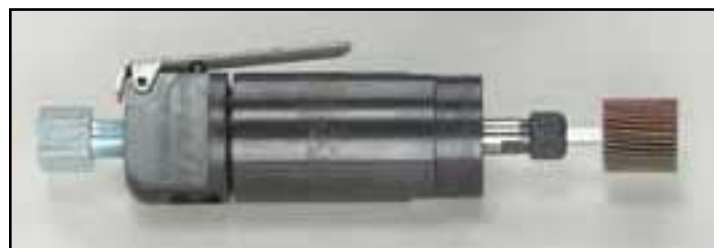
Front exhaust blows chips away from the operator.
